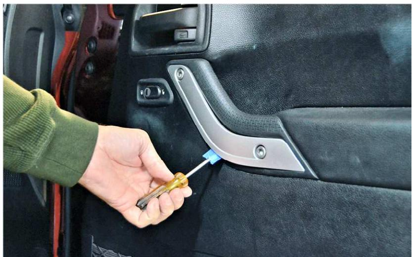
3. Starting at the bottom where you removed the screws from the panel, pull the panel gently away from the door. The goal is to pull the lower half of the panel out far enough to release the pins that secure the panel to the door.
