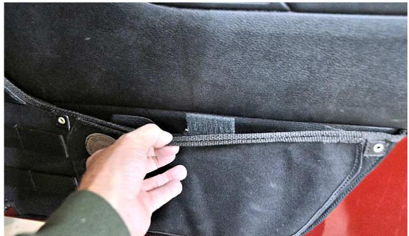
5a. If you plan to use screws to secure the pockets, pull the door pocket up tightly and using a 1/16" drill bit make a hole through one grommet at a time. Insert a screw through that grommet and tighten it into the hole you just drilled. Put screws in the other two grommets the same way.
