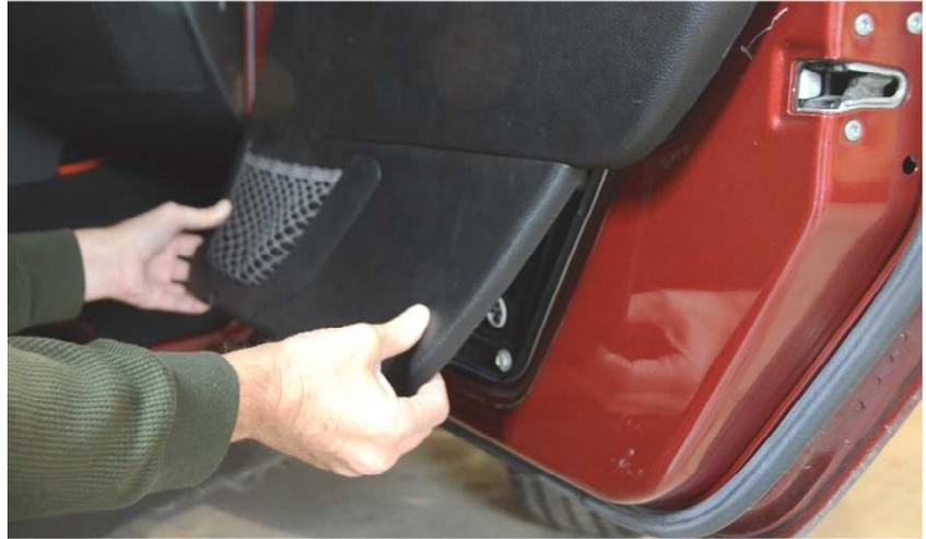
4. Slip the door pocket around the bottom of the door panel, making sure the door pins go through the holes in the back of the door pocket. You will need to reach behind the panel to guide the fabric over the pins so the pins go into the holes in the fabric. Once all the pins are through the holes, pull the panel up tight and push the door panel back in place, being careful that the pins go back in the appropriate holes.
