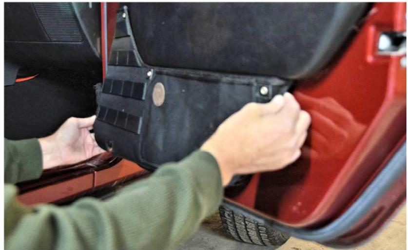
5a. If you plan to use the self-stick Velcro to secure the pockets, put the self-stick Velcro hook patches on the Velcro loop patches on the back of the pockets, pull the adhesive off the Velcro one patch at a time, pull the door pocket up tightly and press the self-stick Velcro onto the door panel.
