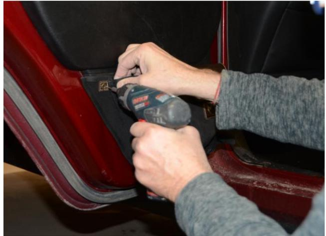
5. Push the panel back in place, ensuring that the push pins go back in the matching sockets in the doors. It will help to look behind the panel as shown at right to guide the pins into the holes. Once the pins are in the holes, push firmly to snap them into place.
