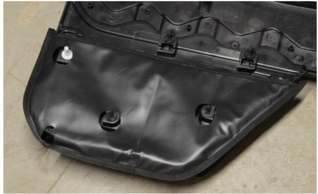
4. Pull the door pocket up tightly and using a 1/16" drill bit make a hole through one grommet at a time. Insert a screw through that grommet and tighten it into the hole you just drilled. Put screws in the other two grommets the same way.
