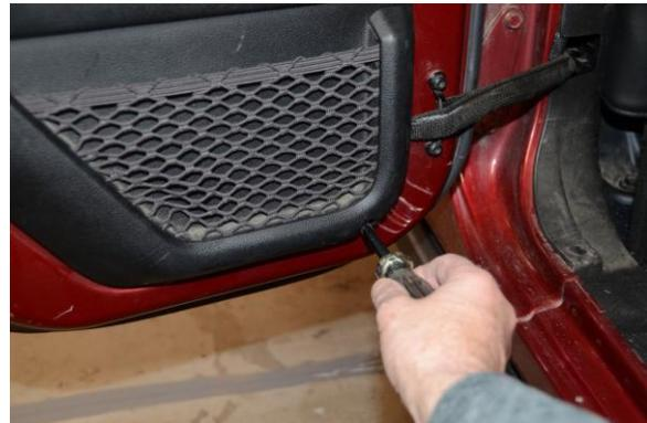
3. Starting at the bottom corner where you removed the screw from the panel, pull the panel gently away from the door. The goal is to pull the lower half of the panel out far enough to release the pins that secure the panel to the door.
