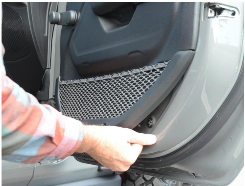
3. Slip the door pocket around the bottom of the door panel, making sure the factory push pins go through the holes in the back of the door pocket. The back view of the panel shows the factory push pins going through the holes in the back of the door pockets. You won't see this view when doing the installation because you won't be completely removing the door panel; this photo is shown to illustrate the push pins.
