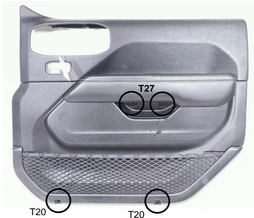
2. Starting at the bottom, pull the panel away from the door. The goal is to pull the lower half of the panel out far enough to release the pins that secure the panel to the door.
