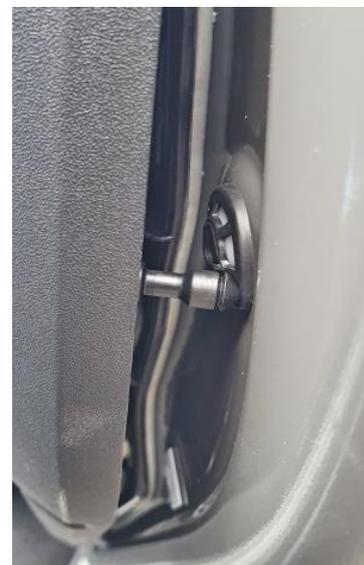
4. Pull the door pocket up tightly and using a 1/16" drill bit make a hole through one grommet at a time. Insert a screw through that grommet and tighten it into the hole you just drilled. Put screws in the other two grommets the same way.
