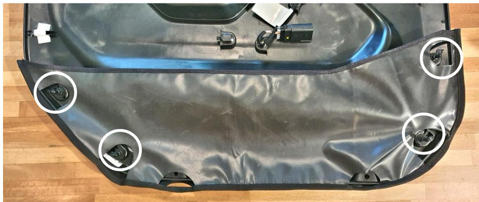
You will need to reach behind the panel to guide the fabric over the pins so the pins go into the holes in the fabric. Once all the pins are through the holes, pull the panel up tight and push the door panel back in place, being careful that the pins go back in the appropriate holes.
